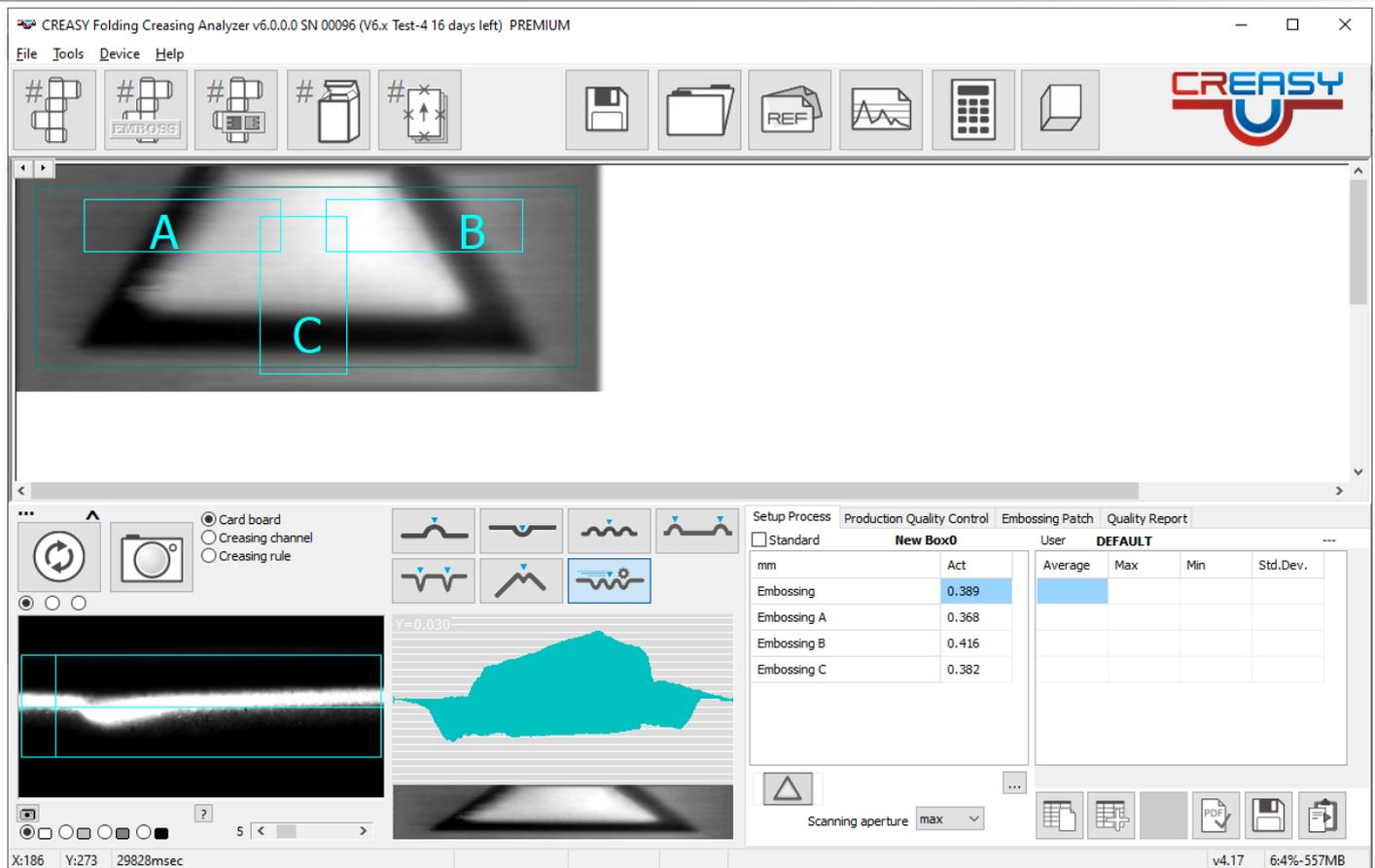
The software will automatically scan over the area and capture the 3D image. There will be measured 3 cross sections A, B, and C as displayed in the main Window.
