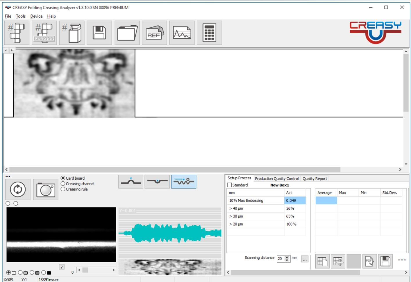
The measurement of embossing test patches does not require the specification of scanning parameters at all. All parameters are selected Automatically. The Software will automatically detect the two embossing areas and calculate depth or height.
