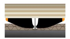
CITO Cushion Crease Plus is mainly used for double and triple flute paper. It is placed on the creasing rule to support compression in a larger area of the corrugated board and to optimise folding behaviour, particularly along the corrugations.
