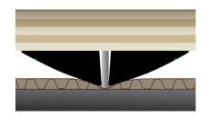
CITO Cushion Crease is used on the creasing rule to support compression of the corrugated board and to optimise folding behaviour, particularly along the corrugations.
