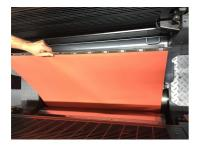
Insert the front side (with the support) into the guide on the gripper striking bar. The PrintGuardPlus is suspended and secured in place by shifting sideways from the drive to the operating side. Make sure that the PrintGuardPlus is locked firmly in place by the this movement and that it cannot be pulled out of the gripper striking bar. Check that the PrintGuardPlus is centred on the cylinder.
