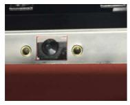
Now inch the machine forwards keeping the PrintGuardPlus under tension at the rear edge. Stop inching forwards when you reach the rear support and can operate the middle hexagon socket screw. If no mistake has been made during the installation of the front, the rectangular cut-outs should be exactly above the rear pins (on the left in the picture). Now hang the rear rail in the pins and release the middle screw with the appropriate
