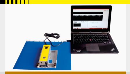
CITO CORRCHECK is an optical, non-contact measuring system for checking the mechanical washboard effect, flute profiles in the case of open flute and the creasing process in corrugated board production.
