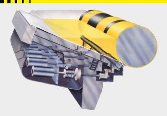
Precisely produced ink duct foils with exact folding ensure fast and uniform application in the ink duct of your printing press. Due to the high stability, the biaxially-orientated foil ensures reliable and uniform ink transport without showing any colour fluctuations or sealing prematurely.
