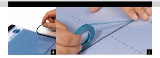
• Remove the self-adhesive supporting foam from the protective paper and affix the 3 mm wide supporting foam circumferentially (at the trim-off area) to the base blanket (fig. 4). Should there not be left any space
