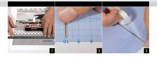
• Measure the print sheet using of the layout sheet in order to determine the necessary settings for making a creasing, diecutting and/or perforating form (fig. 1).
