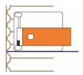
Press down the device with your hand and click the measurement key. The picture will be captured and confirmed with a beep. The Flute profile of the flute in the center of the image will be calculated and the measurement values will show up automatically.
