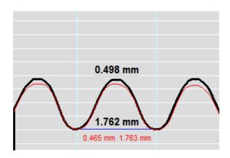
The actual measurement is displayed in black, while the previous measurement is displayed in red.
