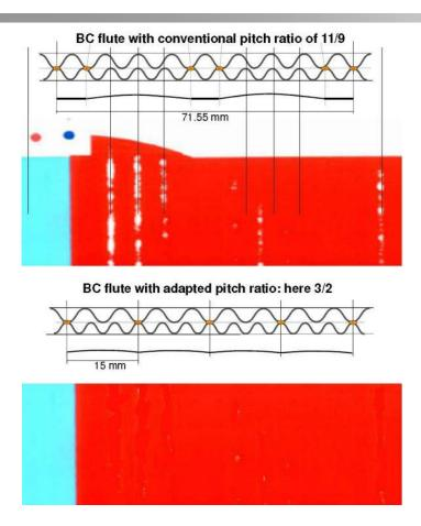
CORRCHECK is an indispensable tool to control the single flute manufacturing process to make sure, height and pitch ratios are correct over the entire corrugated sheet.
