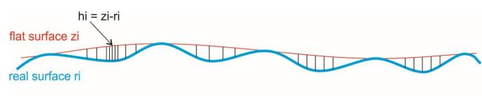
Corrugated card board samples sometimes are not perfectly flat. Therefore the theoretical surface zi (red line) is calculated first. If WBE(1) is selected, this can be a warped line, if warp compensated calculation is not selected, a straight line is assumed. Within one measurement there are calculated approx. 6000 depths  $h_i$  as a difference between theoretical flat surface  $z_i$  and real surface  $r_i$ .
