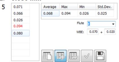
Now measurements in tolerance will be displayed in black while readings out of tolerance will be highlighted in red.
