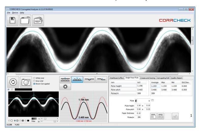
Measurements using a mechanical micrometer will show height information including the material thickness. In order to show comparable measurement values, you can input the material thickness (M) into the proper field during the standard definition.
