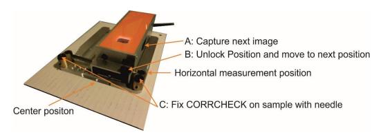
The CORRCHECK hardware is operated with 3 keys:
